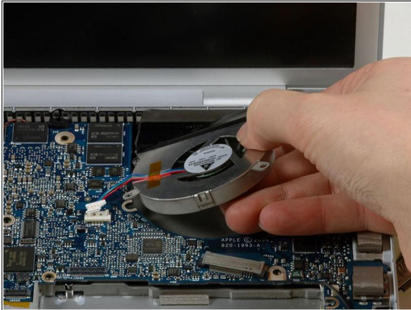
*(i)* It may be helpful to hold the heat sink in place while removing the right fan.
